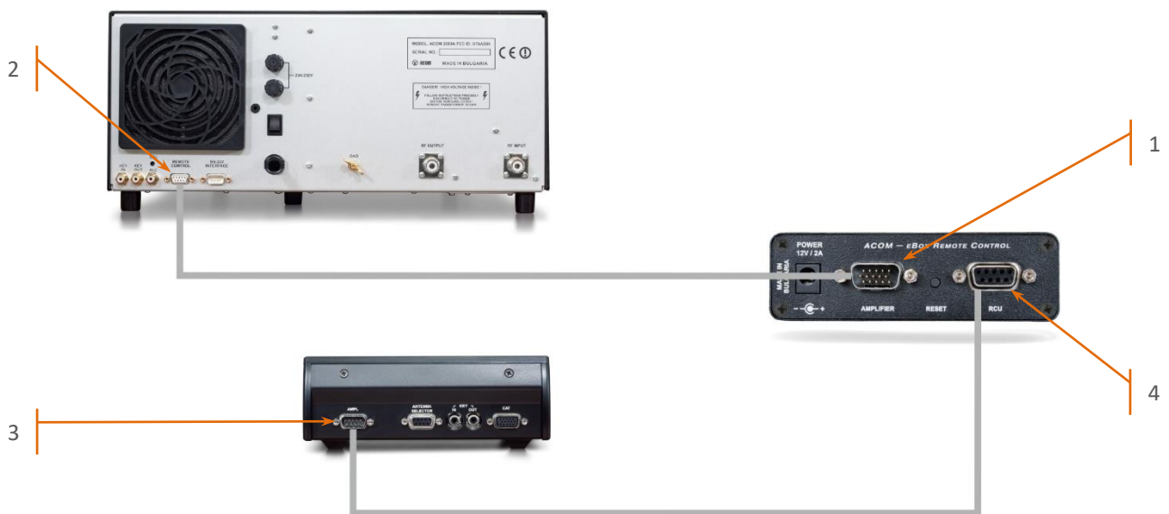
Figure 2-7 eBox to ACOM 2000A connections
